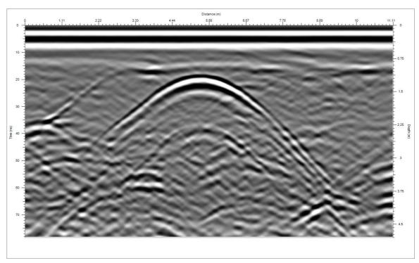
Fig. 3 GCB-200 data showing the tunnel and the water on the sides of the tunnel.
