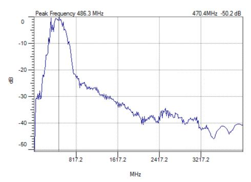
Fig. 2 Power Spectrum of the GCB-500 ground coupled antenna.
