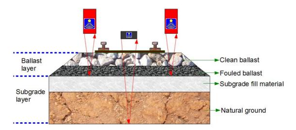
Simplified railroad cross section with GPR antennas positioned over the areas of interest
