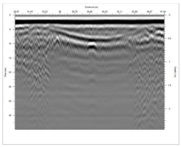
Fig. 4 The concrete slab with the re-bars "hanging" down.
