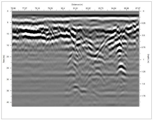
Fig. 9 The small bridge without re-bars.
